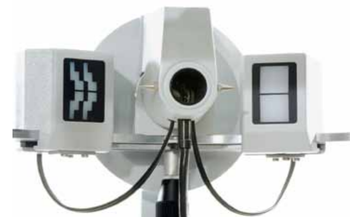
Mire secondo Javal Lines of sight according to Javal
